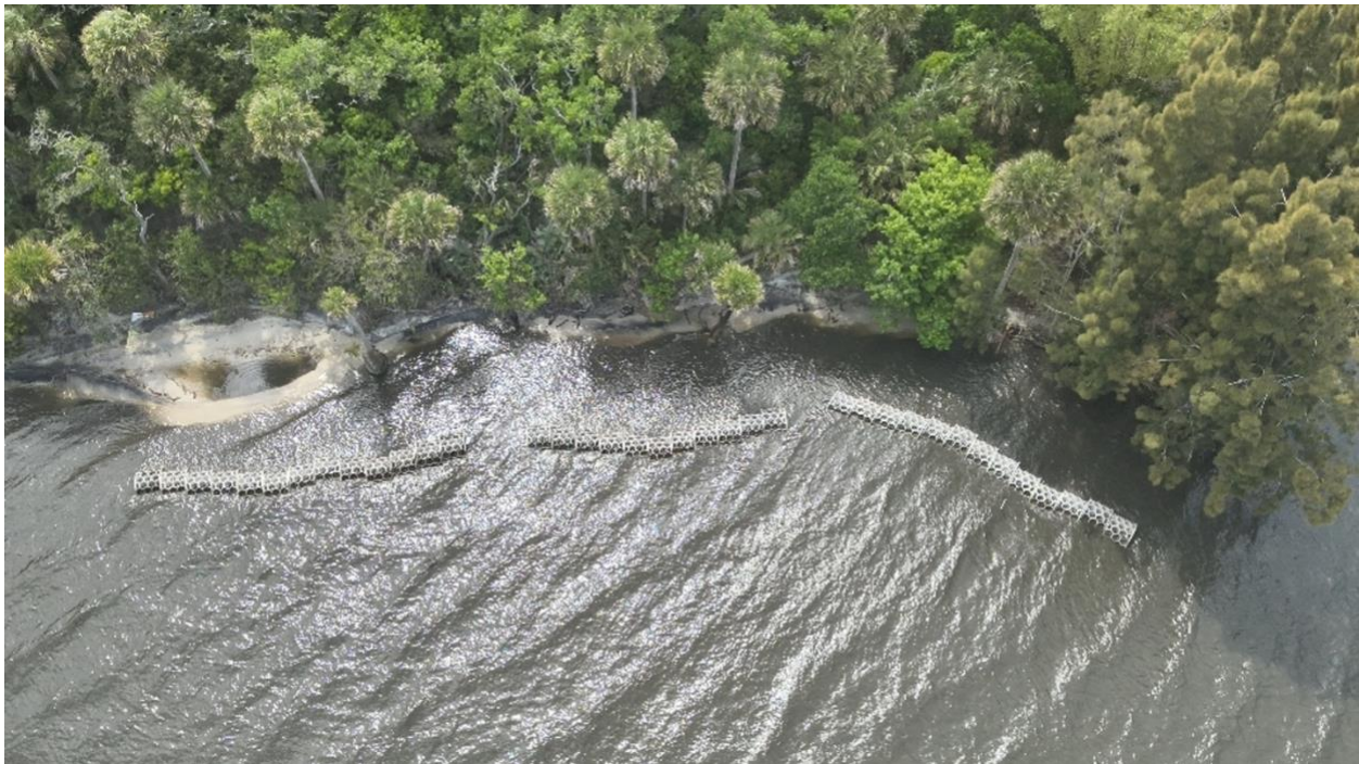
Figure 5. An aerial view of the MRC Reef Arch Deployment taken the day the modules were finished being deployed.
