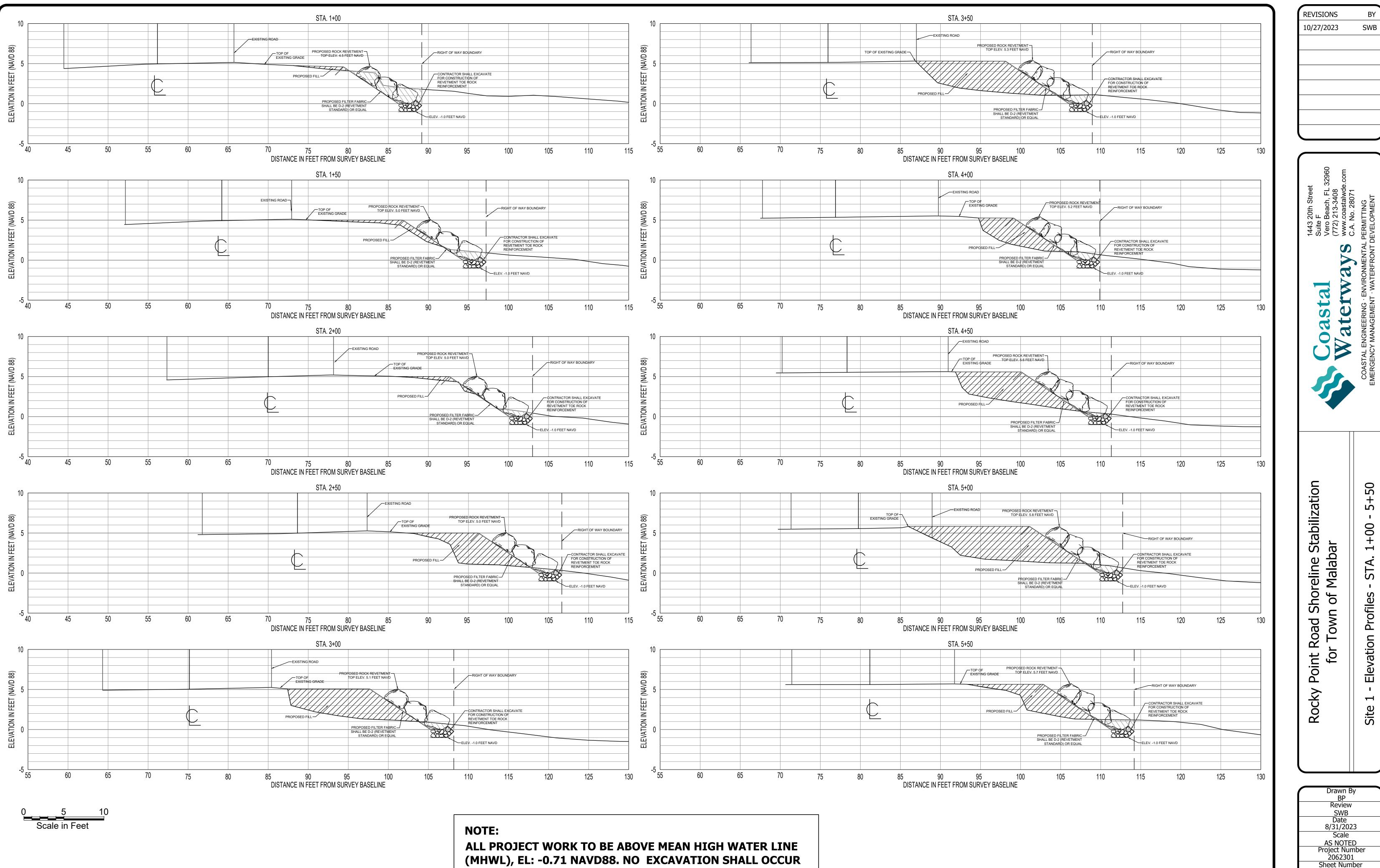
(MHWL), EL: -0.71 NAVD88. NO EXCAVATION SHALL OCCUR **BELOW THE MEAN HIGH WATER LINE.**
